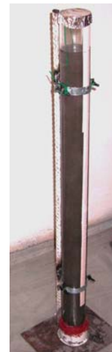
NanoGrout CFG with ZERO BLEED in Wick Induced Test
